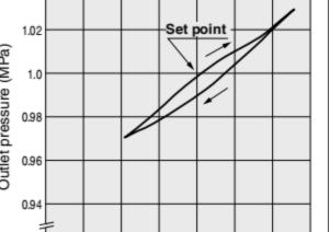
Pressure Inlet pressure: 0.7 MPa Outlet pressure: 1.0 MPa Characteristics
